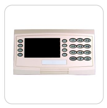
The D1260 Command Center is a SDI Bus compatible device used with 9000 Series Control/Communicators (versions 6.40 and higher). The D1260 features an illuminated keypad, a 4-line by 20-character English language display, and a built-in speaker that emits several distinct warning tones.
